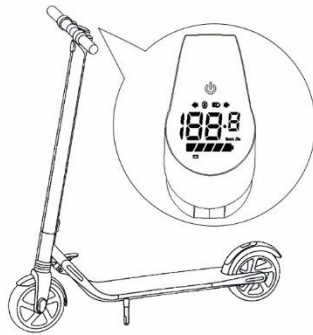
Before use, make sure the vehicle is in good condition, turn on the scooter switch, and check whether the instrument display, power and other functions are normal.
